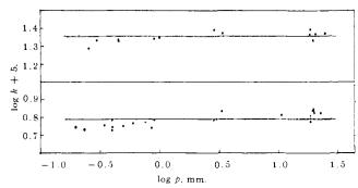
Fig. 2.—Plot of the first-order rate constants vs. initial pressure. The lines have been drawn parallel to the x-axis; top curve at  $366.3^{\circ}$ ; lower curve at  $347.4^{\circ}$ .
